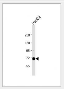
Anti-AFP Antibody (Center) at 1:1000 dilution + HepG2 whole cell lysate Lysates/proteins at 20  $\mu$ g per lane. Secondary Goat Anti-Rabbit IgG, (H+L), Peroxidase conjugated at 1/10000 dilution. Predicted band size : 69 kDa Blocking/Dilution buffer: 5% NFDM/TBST.
